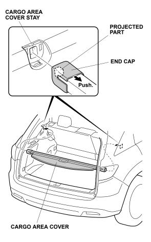
4. Pull out the cargo area cover and secure the two tabs into the channels in the rear side lining as shown.
